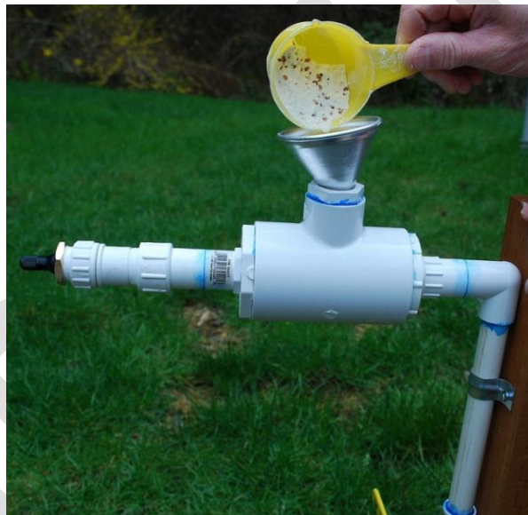
Figure 10. Tilt the volcano on its side and loosely fill the T Slip with eruptive products, such as a mixture of 2/3 cup flour and 1/3 cup birdseed.
