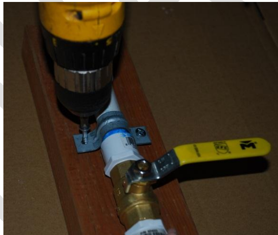
Figure 9. Use screws to securely mount the volcano onto the 2 x 4 lumber using the galvanized straps.
