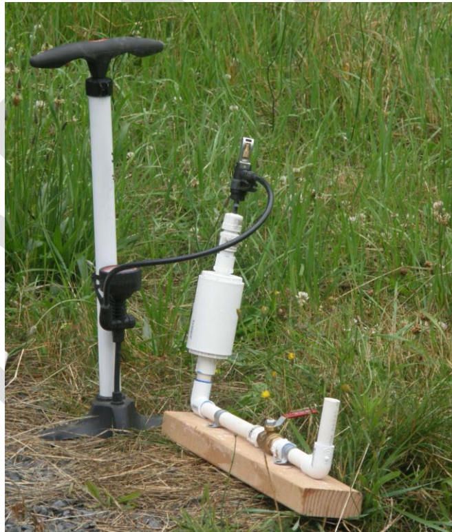
Figure 12. Attach the bicycle pump to the RV Blow Out Plug and pump up the system to 60 psi. Do not over pressurize or the cemented joints may develop leaks. Before conducting the demonstration remind onlookers to stand back 4-meters (12-feet) and warn them to watch out for airborne particles.
