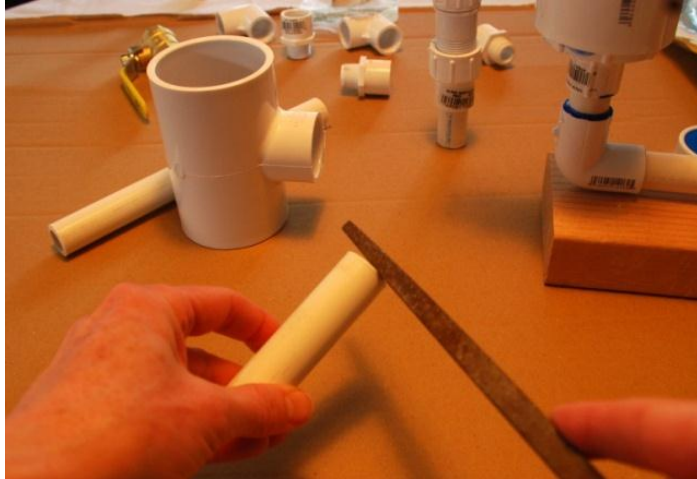
Figure 3. Clean and gently file the ends of the five PVC pipe segments to remove dirt and burrs, making it easier to cement into the fittings.
