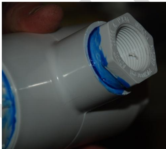
Figure 6. Cement the T-Slip and threaded 1 x ¾ Reducer Bushing.
